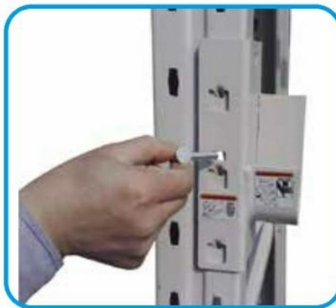
Safety Pin Locks Axle Bracket
